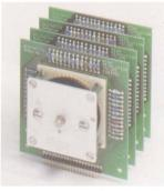
highest grade electronic components are used, including: non-inductive wirewound resistors in the signal path; polystyrene, polypropylene, and Nichicon electrolytic power supply, bypass, and signal capacitors; low noise matched vacuum tubes; glass epoxy dual mono circuit boards; and 20 gauge steel chassis.
